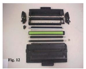
**15.** After cleaning out all the residual toner and inspecting the components, refill with toner and reassemble in reverse order.
