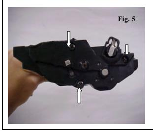
**6.** Detach the side cap by removing the three screws that secure it to the main cartridge body.
