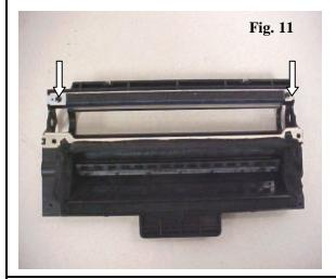
NOTE: The wiper blade assembly in this cartridge is very different than most cartridges. Not only is there a PCR cleaner attached to the blade stamping, the blade itself is little more than an enlarged recovery blade. The toner has a very high transfer rate so there is very little waste in the waste toner collection.
