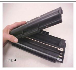
**4.** After removing the screws and clips, simply pull the top cover up to remove.
