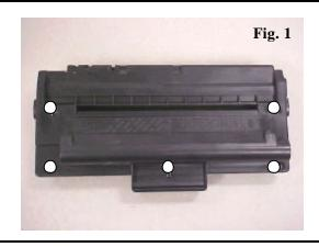
1. Remove the five screws (highlighted area in Fig. 1) on the top cover of the toner cartridge. The cover will not come off, as there are four clips that need to be released for the cover to be removed.
