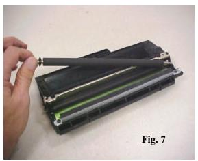
**8.** Once both side plates are detached, remove the PCR.
