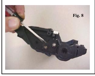
**9.** The developer roller stabilizer plate must be removed to remove the developer roller and OPC. Insert a small flathead screwdriver under the plate and gently pry off.
