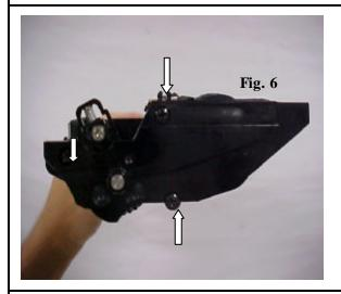
**7.** Remove the side cap on the opposite end of the cartridge using the same instructions.
