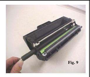
**10.** After removing the developer roller side plate, remove the developer roller by pulling the shaft through the area that was covered by the stabilizer plate.
