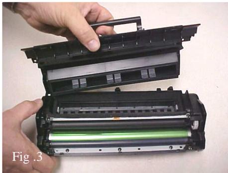
3. Remove cartridge lid. CAUTION, if there is any toner left in the hopper it will spill out. Vacuum out any residual toner from the cartridge interior (Fig 3).
