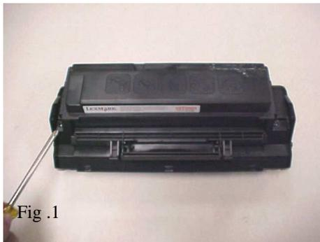
1. Remove the two screws on the top of the toner cartridge shell (Fig 1).
