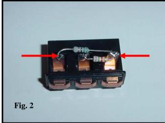
3. Place the contact housing in a secure device. Use needle nose pliers to hold the resistor wire. Heat the solder to remove the resistor on both contacts as indicated (Fig. 3).
