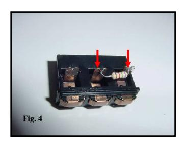
5. Connect the new resistor Oasis Part# SCCHCLP550 (Fig. 5) to the 2 contacts tabs (Fig. 5a).
