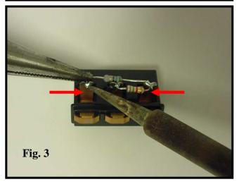
4. Once the resistor is removed, clean both contact points of remaining solder.
