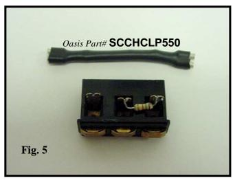
6. Once the resistor is connected to both contacts, snap the housing back into the cartridge (Fig. 6).
