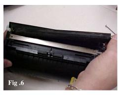
7. Remove the hopper cap and yield wheel than clean the hopper of all residual toner using compressed air or a vacuum. Inspect the developer roller sealing blades. If they are loose or damaged replace them. Thoroughly clean the foam toner delivery roller with compressed air being careful not to damage the sealing blades. Using a cotton swab, clean the underside of the metering bar thoroughly of any residual toner (Fig 7).
