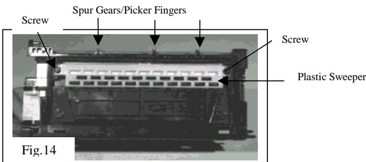
7. The plastic sweeper can be removed for cleaning if you choose, however removal isn't necessary. Compressed air will clean the sweeper appropriately.
