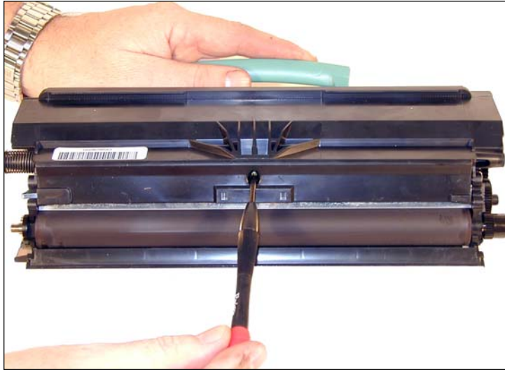
13. Re-install the developer roller cover and screw.
