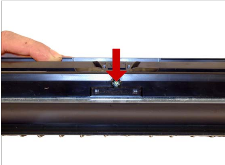
1. Remove the developer roller screw & cover.
