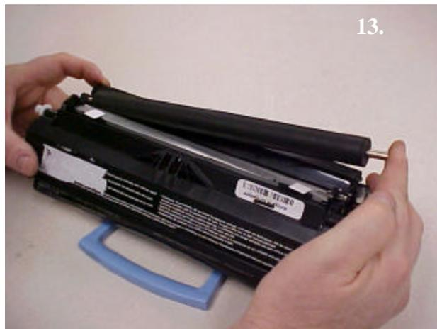
1. To remove the developer roller from the toner hopper, gently push the shaft from the geared end of the developer roller toward the fill cap side of the toner hopper.
