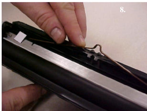
1. Before you can remove the developer roller, it will be necessary to remove the doctor bar tension spring.
