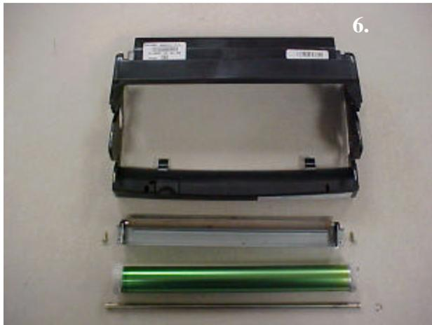
1. After removing all old toner, replace all of the worn components.
