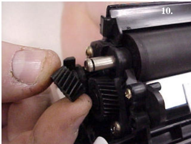
1. After removing the c-clip from the developer roller drive shaft, remove the small helical drive gear from the shaft and set it aside.
