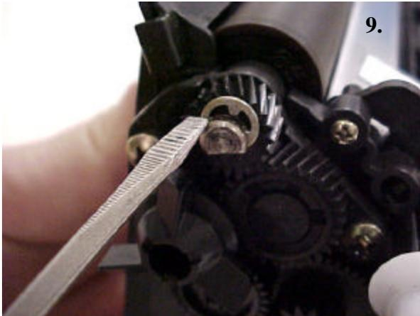
1. To remove the developer roller, it is necessary to remove the e-clip from the developer roller shaft.
