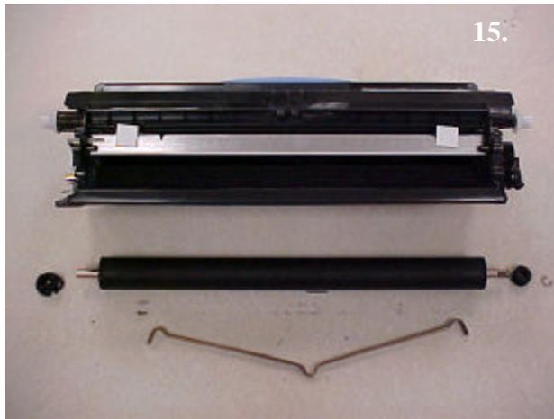
1. Using compressed air and a vacuum, clean all of the OEM toner from the toner hopper.
