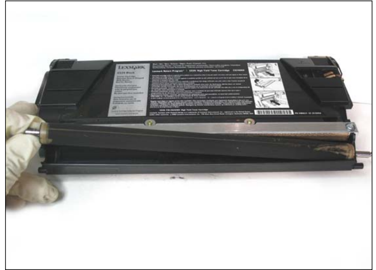
12. Remove the DVR roller.
