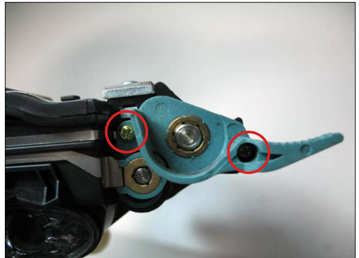
10. Remove the small DVR support plate on the contact side by removing the two screws holding it in place (marked with circles).
