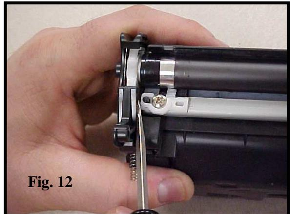
13. Remove the end cap. During reassembly of the hopper section, the two screws will be sufficient to secure the end cap to the toner section (Fig.13).
