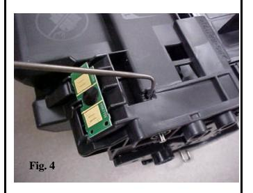
4. Push the pins out enough to be able to place a pair of pliers on the pin to fully remove it, once it is free from the internal housing. Once the pins are removed, you can separate the cartridge halves.
