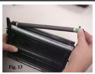
13. Carefully remove the magnetic roller by first lifting the end of the roller and then gently pulling it to the right. Note the location of all peripheral components on the mag roller (bushings, brackets, etc.). Use compressed air to remove all residual toner from the surface of the mag sleeve and inspect for damage. Set the mag sleeve aside or replace, if necessary.
