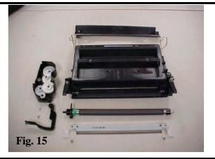
15. Clean the toner hopper thoroughly with compressed air or vacuum. Fill the hopper through the mag opening. Clean or replace components and re-assemble the toner hopper in reverse order.
