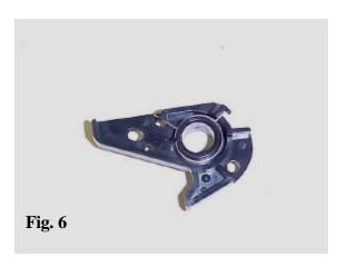
6. Over the drum axle is the cartridge sensor tab. When removing the drum, the sensor tab is removed. This step shows the spring orientation when it is reinstalled.
