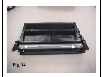
14. Remove the two (2) screws holding the doctor blade in place.
