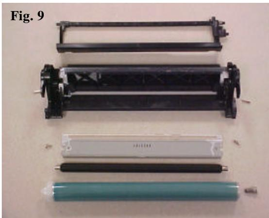
**16.** Clean the waste hopper section with compressed air.
