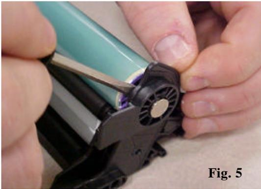
**8.** To remove the OPC, insert a small flat-head screwdriver between the end of the OPC and the inner cartridge wall.
