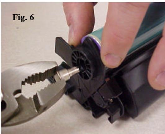
**10.** Grab the exposed head of the OPC axle with a pair of pliers.
