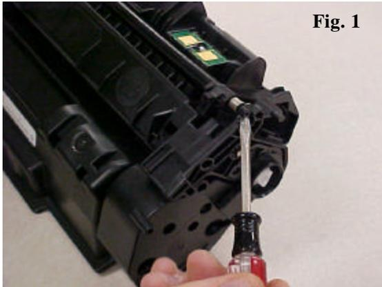
1. Before separating the cartridge halves, remove the OPC protective shutter.
