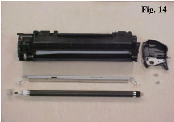
**23.** After cleaning out all of the toner from the toner hopper, be sure that the electrical contacts are clean and reassemble in reverse order.
