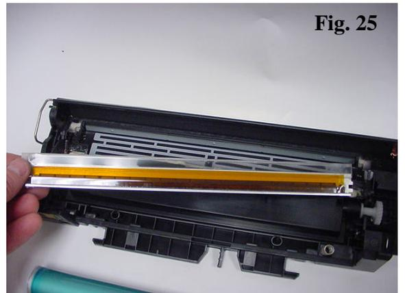
26. Clean the waste unit of all residual toner using compressed air. Clean and or replace all cartridge components. Use caulking on the back edge of the metal stamping of the wiper blade once replaced. This prevents leaking from the waste bin. Clean and re-apply all contacts with conductive grease. Reassemble in reverse order (Fig. 26).
