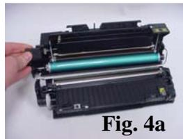
5. Remove one screw from the contact side end cap of the toner hopper (A). Use a small flat head screw driver to release the locking tab located on the top of the end cap (B). Remove the end cap (Fig. 5).
