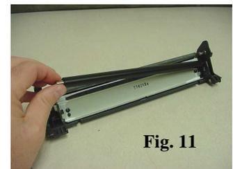
9. Remove the two screws that secure the wiper blade (Fig 12). Remove the blade and replace if necessary. Remove all residual toner from the waste bin. Check Mylar recovery blade and ensure that it is not creased or damaged. Clean or replace PCR and OPC and reassemble in reverse order.
