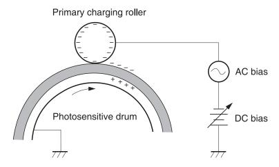
In the **first** step, the Primary Charge roller (PCR) places a uniform negative DC Bias voltage on the OPC drum surface. The amount of the negative DC Bias placed on the drum is controlled by the printer's intensity setting. This process is part of the latent Image formation block.
