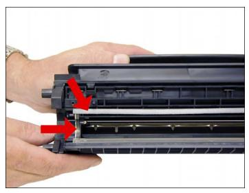
27. Note the magnetic seals on the MRS and the DB sealing foam. Make sure both are clean.
