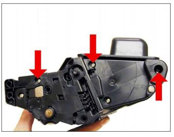
41. Install the remaining three screws on the left end cap.
