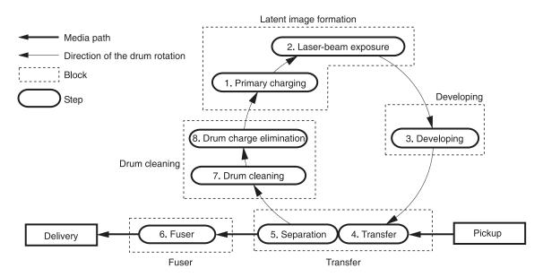
The image formation process consists of 8 steps which are split up into five functional blocks.
