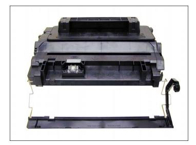
4. Remove the metal bar from the left side, and remove the entire drum cover assembly. Make sure you put the spring in a safe place.
