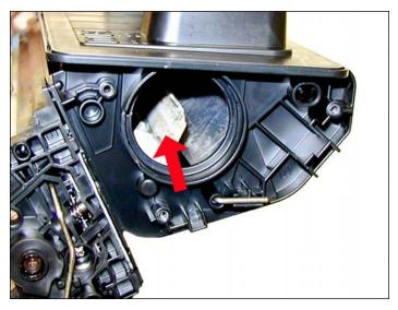
30. Unlike the HP-4300 series where there are three separate mixing blades in the toner hopper. These cartridges just use one large mixing blade inside the toner hopper.
