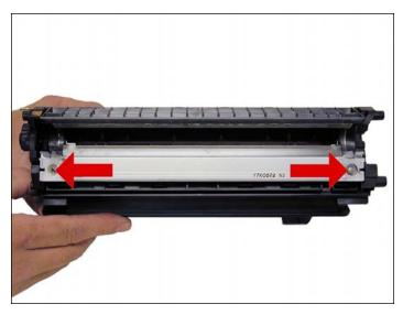
31. The upper mag. roller section of the toner hopper is different in that is "Floats" on a series of foam seals. The upper half can be removed from the hopper, but some of the seals will be destroyed. This may become necessary in order to seal the cartridge we will keep you informed as our testing continues. The foam isolates the mag roller from the vibrations of the mixing augers, and allows smoother prints.
