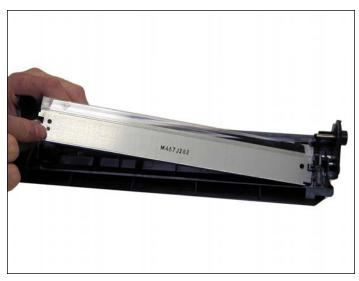
13. Remove the wiper blade from the cartridge and clean out the waste toner.
