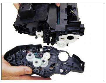
7. Remove the right and left side end caps from the cartridge. Note that the gears do not come off the gear (right) end cap.
