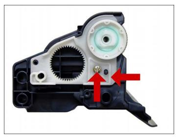
20. Install the white plastic drum bushing and screw. If the OEM drum grease is dirty, clean it off with alcohol, and replace with white lithium grease.
