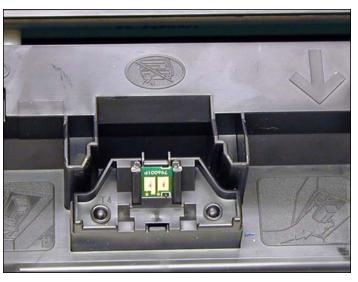
45. Remove the old chip from the top of the cartridge by slicing the melted plastic off with a sharp X-Acto knife. Replace the chip, then lock in place with a small dab of glue from a hot glue gun. Replacing this chip will enable the toner low functions of both the cartridge and the machine again.
