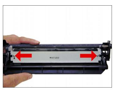
15. Install the new wiper blade and two screws.
