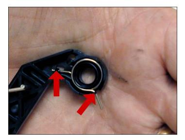
42. Install the spring into the drum cover arm as shown. Pull the upper tail of the spring until it fits into the notch in the arm hub.
