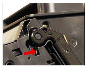
44. Install the arm onto the cartridge. Pull the arm fully back to release the spring from the notch. Check to make sure the drum cover operates properly.
