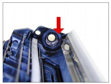
29. There are HP-4000 style magnetic roller bushings on each side of the roller. While these are holding up well in our initial tests, this may be an area where wear will cause banding. One will stay in the hopper, and one comes off with the mag. Roller assembly.
