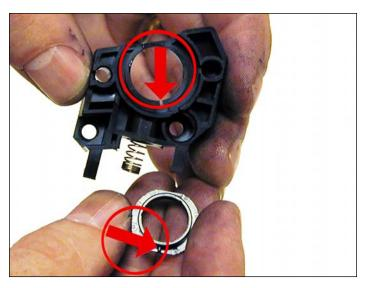
34. Remove the right side small bushing from the magnetic roller sleeve and install it onto the holder. Make sure the tab on the bushing aligns with the slot in the holder.
