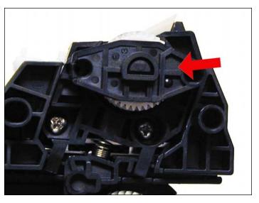
37. Install the keyed MRS cover. Make sure that the keyed hole in the cover matches the keyed end of the magnet in the MRS assembly.
