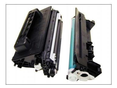
8. Separate the toner hopper and waste chamber.
