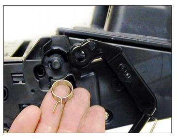
3. On the opposite side of the cartridge, carefully pry off the drum cover plastic arm. The spring will probably pop off, take care not to loose it. We will go over the installation at the end of this article. Remove the drum cover assembly.
