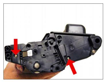
39. Hold the two sections of the cartridge together, and install the left (Contact side) end cap. Install a screw in the waste and supply sections to hold everything together.
