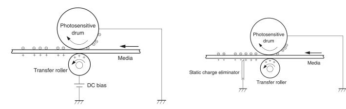
In the **fourth** step (transfer block) the toner image is then transferred to the paper as it passes below the drum by the transfer charge roller, which places a positive charge on the back of the paper. This positive charge causes the negatively charged toner on the drum's surface to be attracted to the page. The small diameter of the drum, combined with the stiffness of the paper causes the paper to peel away from the drum.
