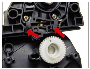
35. Install the holder 2 screws and spring. Make sure the screw holes line up, and that the two locking tabs on the bottom of the holder are in the correct place.
