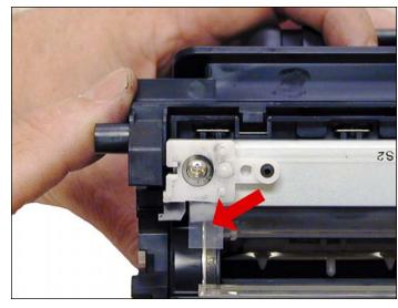
25. Remove the two doctor blade screws and the doctor blade. Note the clear plastic strip that covers the DB screws. Slide the screwdriver under the strip. Be careful not to damage the strip!
