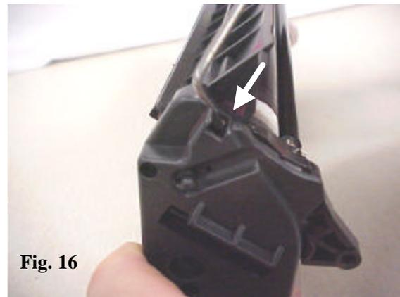
17. Remove the cap from the end of the toner hopper unit.
