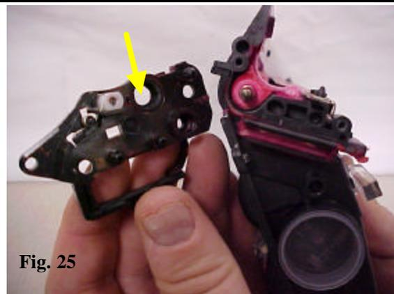
26. Remove the two screws that secure the doctor blade to the toner hopper.
