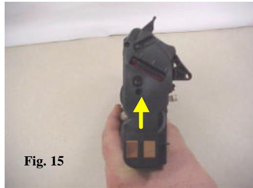
16. Once the screw is removed, the end cap is still held in place by a locking tab on the top of the end cap. Release this tab to remove the cap.
