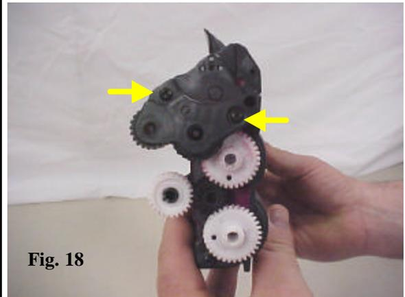
**19.** Remove the end cap. Remove six gears and note the orientation of them for reassembly.
