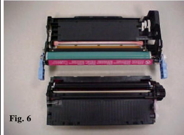
7. Starting with the drum section, remove the small screw from the cartridge handle where the tension spring is located.
