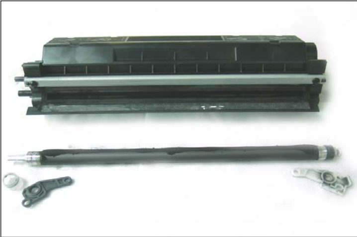
26. (a) Remove the stabilizing arm and mag roller bushing from the gear side (left) of the roller.
