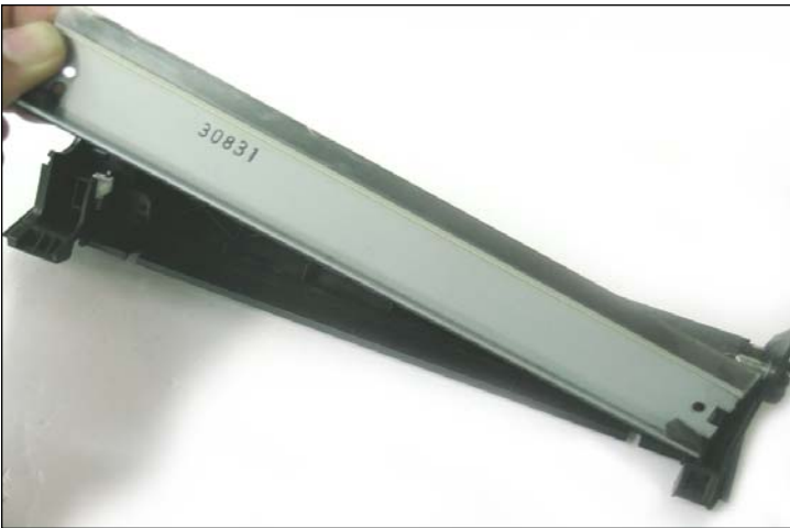
15. Remove the wiper blade and empty the waste toner. Clean the waste hopper using dry compressed air or vacuum.
