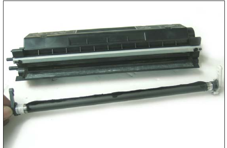
25. Lift the mag roller away from the toner hopper.
