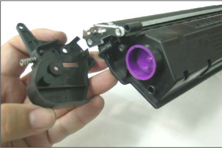
24. Remove the contact end cap to reveal the toner fill plug inside.
