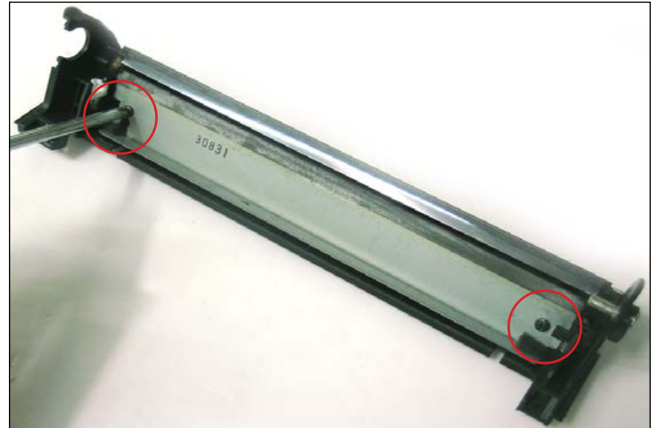
14. Remove the two screws that hold the wiper blade in place.
