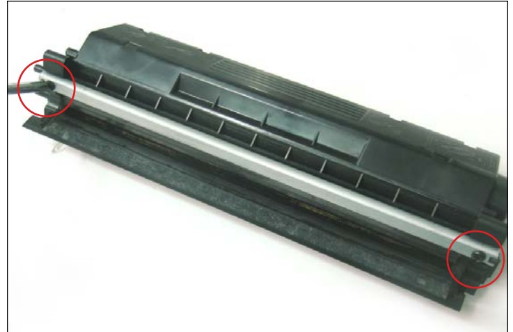
27. Remove the two screws holding the doctor blade as shown. Remove the blade and clean using a lint-free cloth and alcohol.
