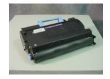
1. Remove one screw securing the spring loaded drum shutter actuator arm. Remove the spring from the actuator arm. The actuator spring is tension loaded into the actuator arm and may dislodge and become lost.
