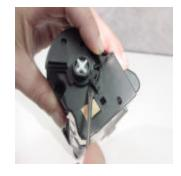
4. Remove the two screws that hold the side plate on. After removal of the side cap inspect it for damage and clean all contacts with 99% Isopropyl Alcohol and set it aside.
