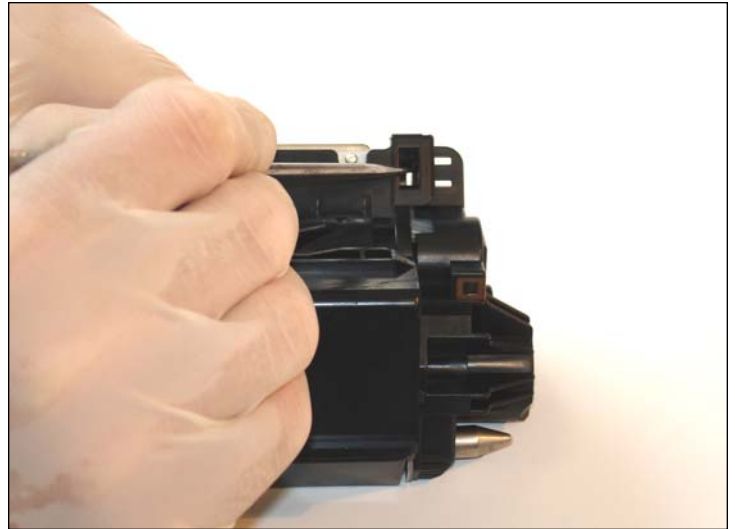
8. Push carefully the black end cap tap as shown using a straight hook tool.
