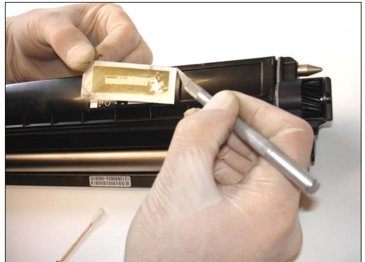
40. Cut the label using a X-acto knife.
