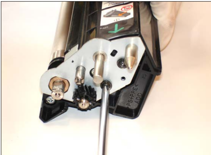
11. Remove the screws from the metal gear plate.
