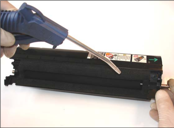
21. Use compressed air to clean the toner chamber and the cartridge. Make sure the foam seal around the slot is clean and not damaged. Pay attention to not damage the sealing foam.
