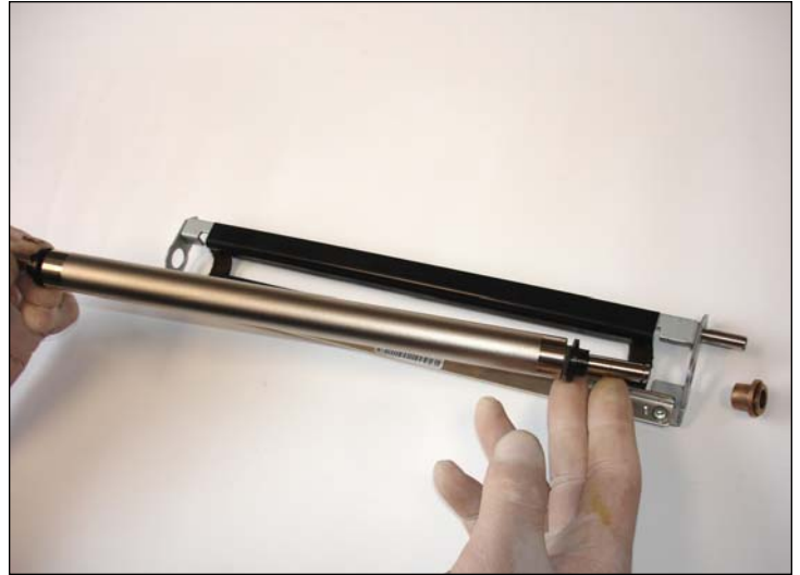
30. Place the develop roller and reassemble its parts in reverse order.
