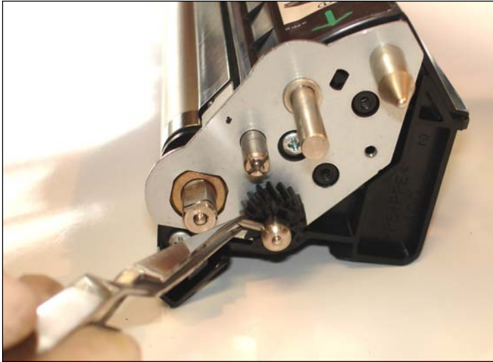
13. Push the gear until you could release the pin from inside. We recommend using a flat needle head tweezers.
