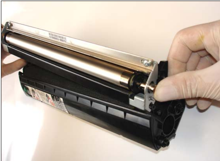
31. Put the whole develop frame on the cartridge. It should fit the previous position on the sealing foam.
