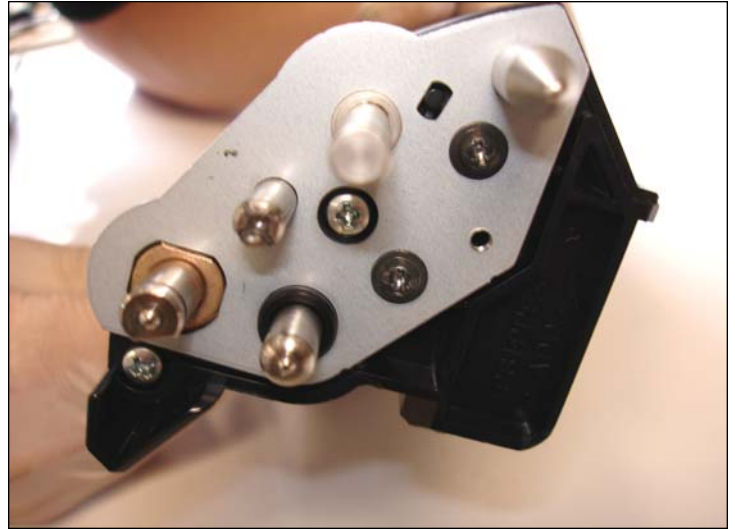
34. Place the metal gear support endplate until it fits properly with the previous installed bearing.
