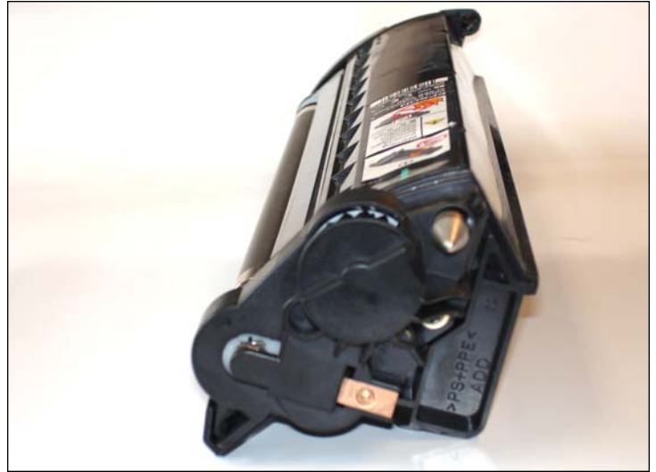
2. Toner unit gear side view.
