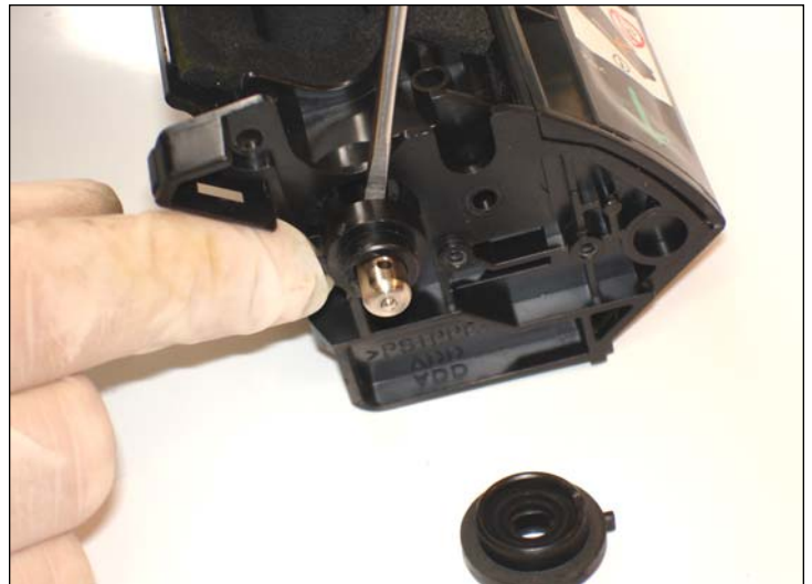
20. Remove the black add roller bearings from both sides.
