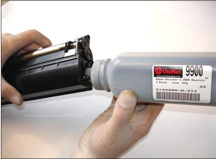
37. Fill the hopper with the specific toner and place the fill cap.
