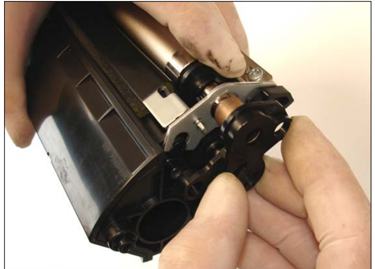
32. Place the black develop end cap on the right side as shown and screw it.
