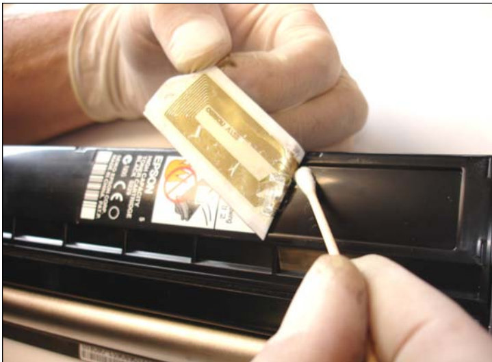
39. Remove the OEM label where the chip is placed as shown.
