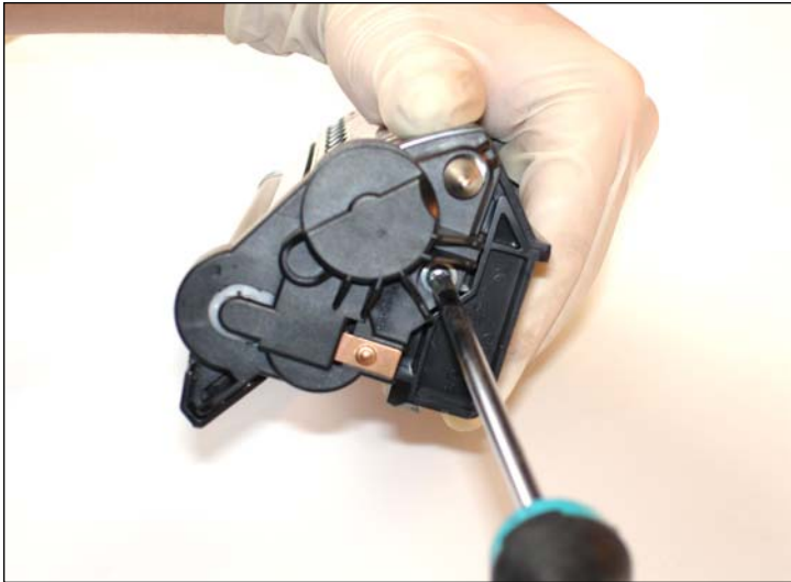
7. Take out the other side's screw by means of a Phillips screwdriver.
