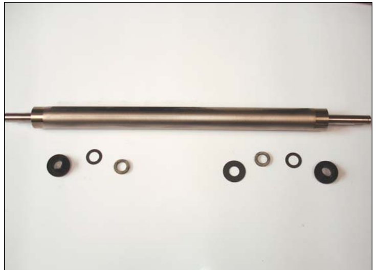
24. DVR washers & bushings should be assembled as shown.
