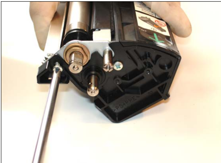
15. Remove the two Phillips screws which ensure the correct position of the DVR frame. Note the thread is different.
