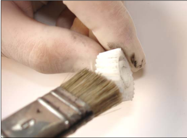
29. Clean the gears with a cut hair brush with isopropyl alcohol to avoid a blocked cartridge.
