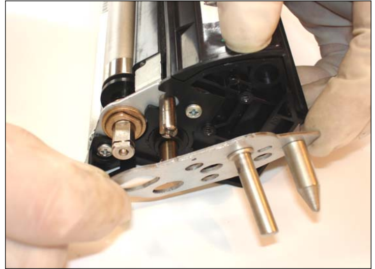
14. Release the metal gear endplate.
