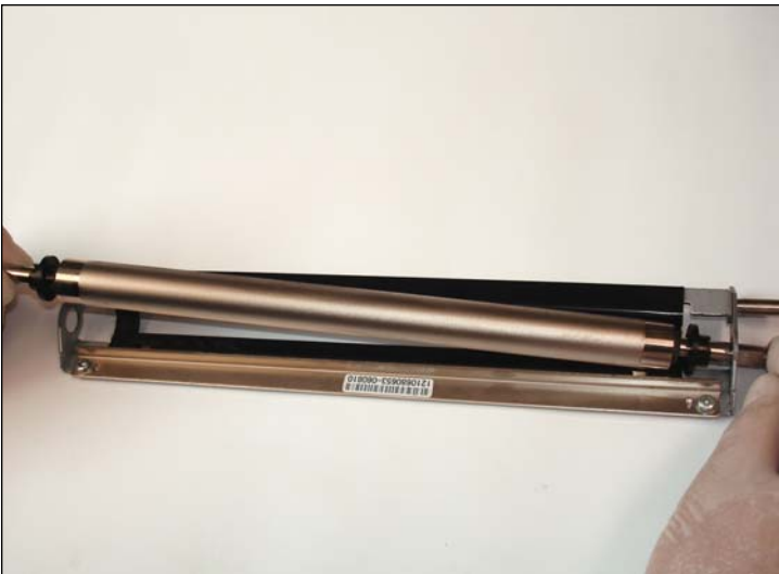
23. Remove the develop roller by lifting it from the left side.
