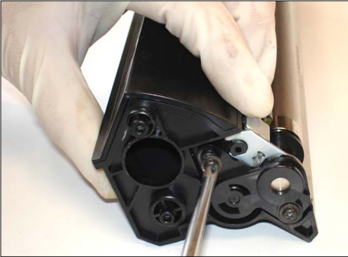
17. Unscrew the following two black Phillips screws from the fill cap side.
