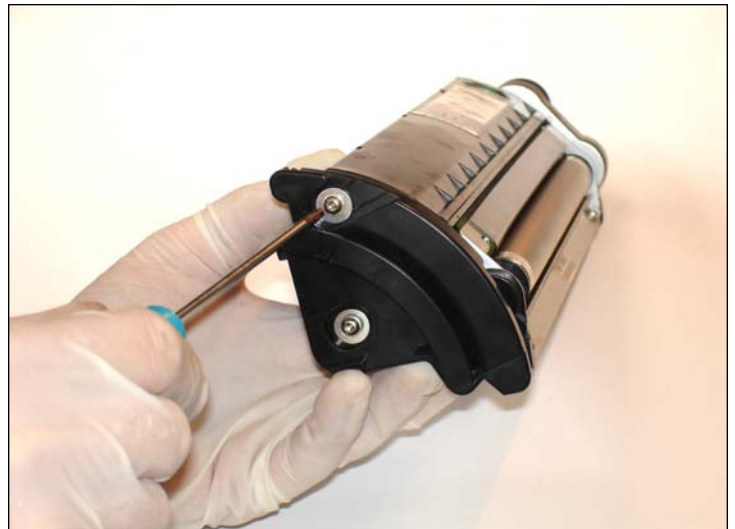
4. Remove the two torx security screws from the colour cover side using a Security torx screwdriver.
