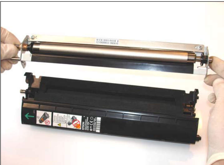
19. Free the whole develop frame carefully.
