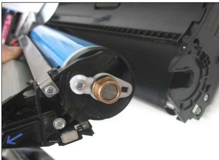
7. Carefully separate the OPC drum from the waste hopper.
