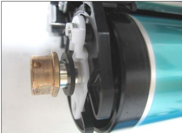
9. Slide off the copper and black bearings (shown) to access the plastic drum axle support.
