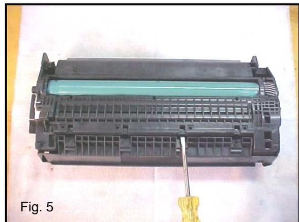
6. Separate the two cartridge halves.
