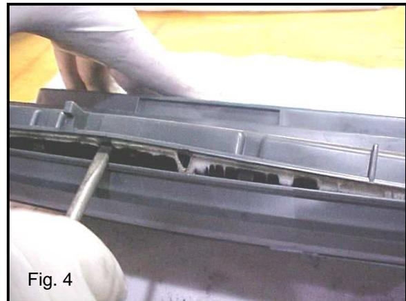
5. Use a flat-head screwdriver to release the 4 tabs located on the bottom of the cartridge (Fig. 5). Some of the tabs may break off. We will use screws to fasten where the tabs break off during reassembly.
